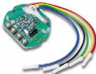
2/4-channel battery concealed transmitter, FS20 S4UB Concealed transmitter for location independent connection for up to four installation sensors and control of 2/4 functions. Battery with 10 years service life. Order no.: 17-566-06
